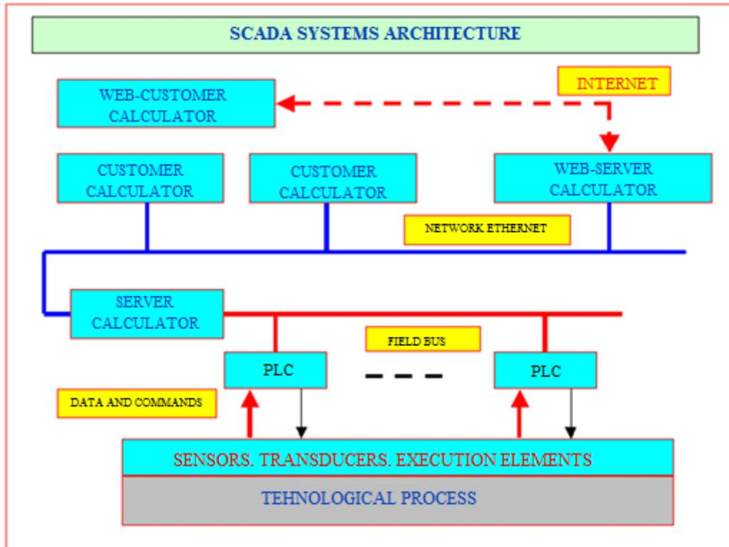
Fig.2. SCADA systems architecture
