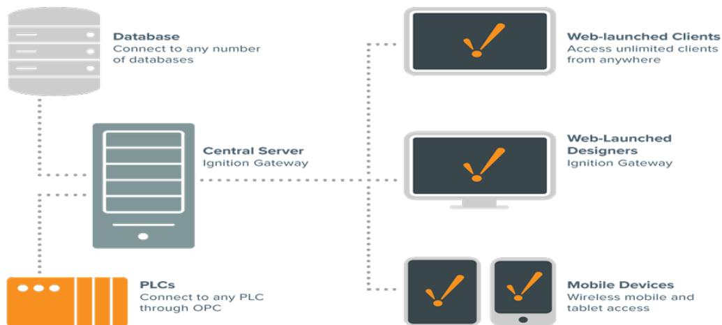
**Fig. 3.** Ignition SCADA Architecture
